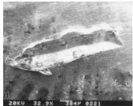
Fig. 3 Typical morphologies developed after impact scratching the electrodes of 2014 aluminum alloy, which have been solutionized at 540 °C for (a) as-received condition, (b) 5, (c) 10, and (d) 20 h
